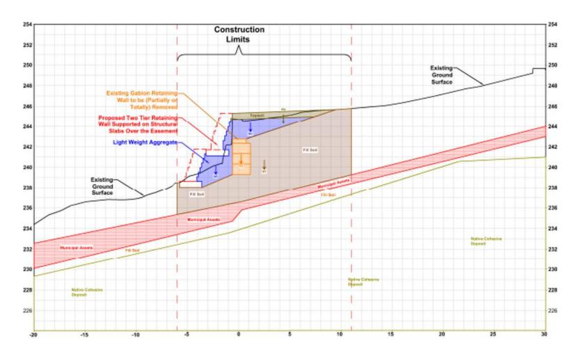
Figure -2 Easement Cross Section E-E' Station 0+12.5
