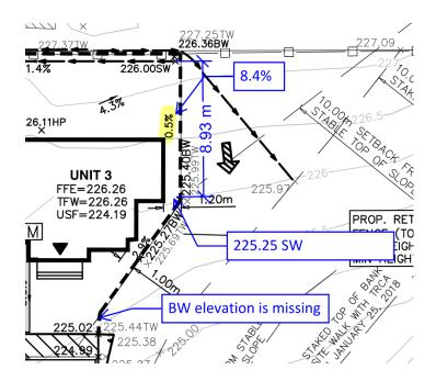
h. The Erosion and Sediment Control Plan (Drawing No. C05) still does not demonstrate how the NE corner of the development will drain towards the sediment trap. The swale elevations and sediment trap inverts for inlet and outlet are also not shown. The ESC plan should be revised prior to commencing any earthworks.
